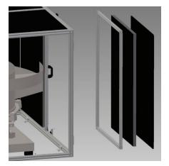
Attica Automation sound enclosure construction is made from these three materials: Extruded aluminum frame, 1-1/8" Soundproofing composite and 1/4" plastic exterior panels.
