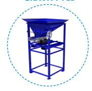
The AF-G100 is a gravity fed bulk feeding system that incorporates into each of our inspection systems. Designed to be loaded with a fork lift, this system can be controlled through the system, or it can be setup as an independent feeding system.
